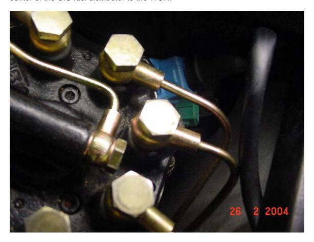
Surround the WUR with paper towels. Loosen the 14mm banjo bolt fitting from above with socket wrench. Two copper crush washers seal the fitting from both above & below; try not to lose the lower ring into the engine valley. A small amount of fuel will spill from the line (residual pressure from overnight).
