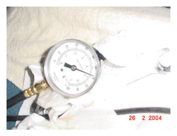
Turn ignition off. Pressure will rapidly fall to approximately 40psi and hold. Allow car to stand for 20 minutes; the accumulator should hold a minimum of 3-3.5 bar (approximately 40psi) for minimum 10-20 minutes if functioning properly and injectors are not leaking.
