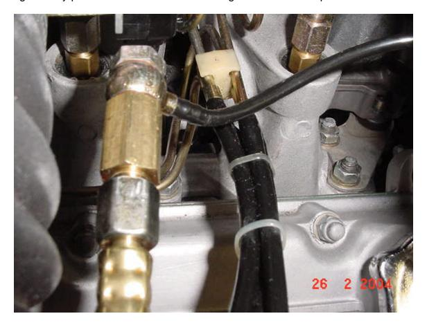
Next, attach a second adaptor to the input port of the WUR (15mm in my set). Connect the other main tester hose (side with valve) to this fitting:
