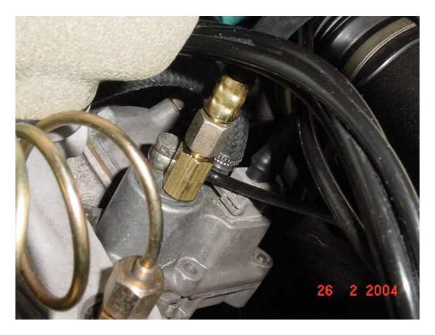
My pressure gauge line then attached to the T-fitting using a snap-collar type lock:
