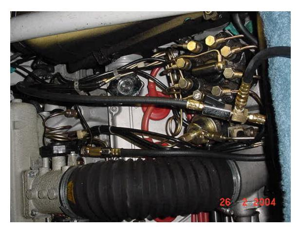
Remove the blue fuel distributor safety switch connection from the rear of the mixture control unit to allow the fuel pump to run without actually starting the engine. I also disconnected the cold-start injector in case it was signaled, but this is probably unnecessary. Temporarily disconnect the input signal harness to the WUR:
