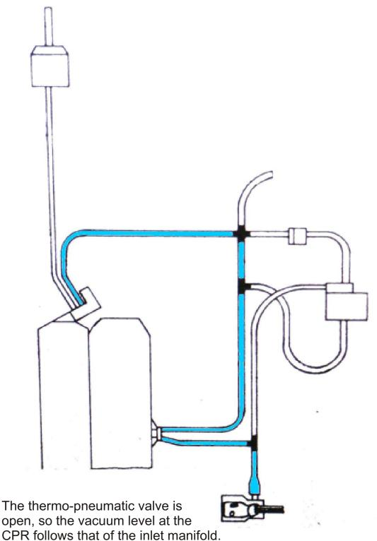
Enrichment will happen as soon as the throttle is partially opened and the inlet manifold vacuum drops.
