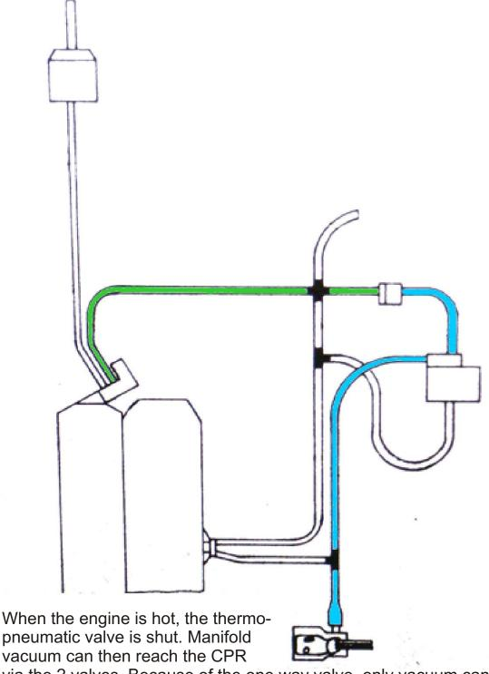
via the 2 valves. Because of the one way valve, only vacuum can pass - not boost pressure. Maximum attained manifold vacuum is then held on the CPR (resulting in a leaner mixture) all the time until the WOT switch is activated.
